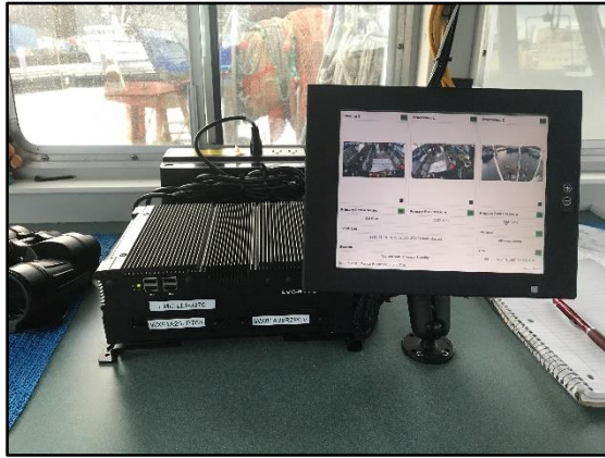
A computer monitor displays camera images of an electronic monitoring system on board a catcher vessel.
