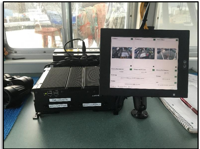
Computer monitors display camera images of an electronic monitoring system on board a catcher vessel.
