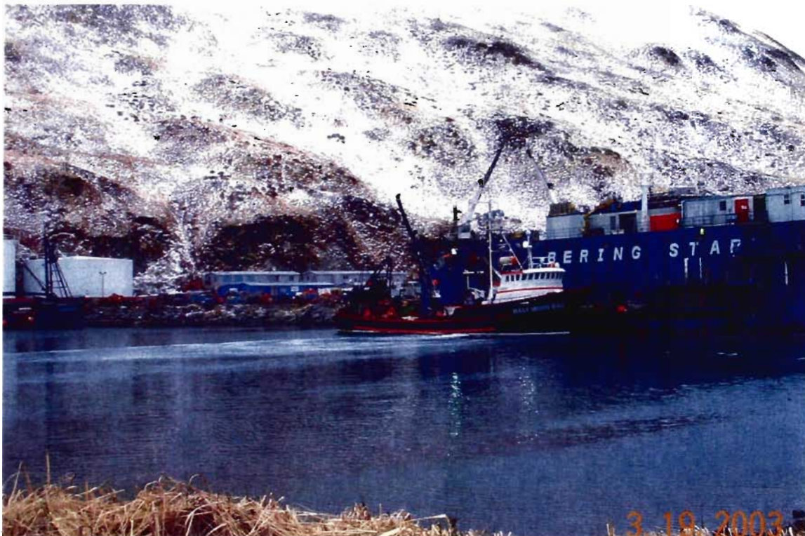
Figure 5. A trawler offloading its catch at the floating processor at the head of Dutch Harbor. This vessel is being unloaded by a brailer since the floating processor is not set up to use a vacuum line to offload the fishing vessels. The white discharge is from the vessels hold. The floating processor is typically moored in its present location for the entire winter where it discharges waster material to the outside of the spit through an underwater outfall line.
