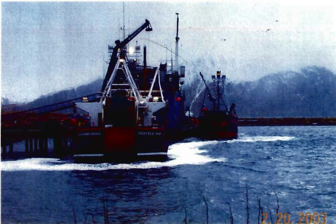
Figure 4. The fishing vessel on the right is offloading its catch and pumping its hold resulting in the white foam. The trawler in the foreground is tied up and is not contributing to the discharge.
